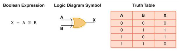
**Tip:** When memorizing the gates, focus on the expressions and the diagram symbols. While the truth tables are extremely helpful for understanding the relationship between the inputs and outputs, they can be quickly reconstructed by substituting the variables in the expressions with the possible combinations of 0s and 1s.
