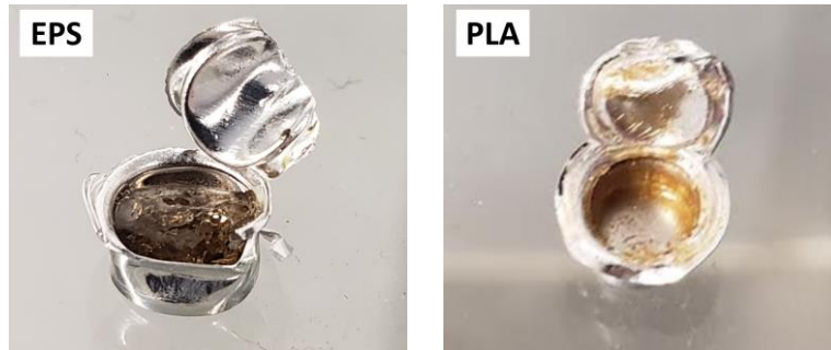
Fig. 24. Residues inside DSC sample holders after the test. After the test, the EPS sample holder retains most of the polymer mass, while the PLA sample has degraded mainly by evaporation.
