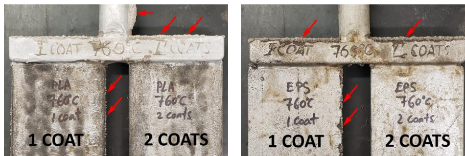
Fig. 10. Melt infiltration and river surface, 750 °C, top-down filling: PLA foam casting (Left) and EPS foam casting (Right).
