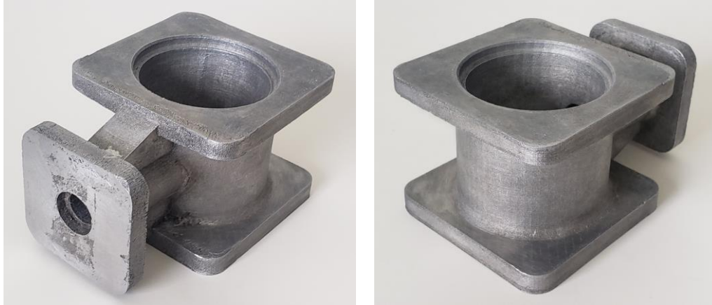
Fig. 22. GD&T (valve body) casting from 3D printed PLA foam pattern, 800 °C, top-down filling.
